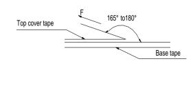
The force for tearing off cover tape is 10 to 130 grams in the arrow direction under the following conditions (referenced ANSI/EIA-481-C-2003 of 4.11 standard)
